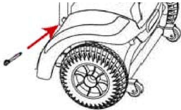
Tighten the bolt near the top of the seat tube with the included Allen wrench.
