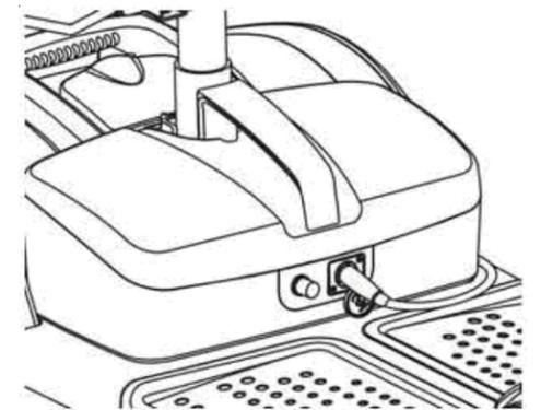
Full charging normally takes 6-8 hours, but can take as many as 10 hours depending on the batteries' charge level when starting and the ambient temperature.
