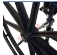
24-inch quick release rear wheels
