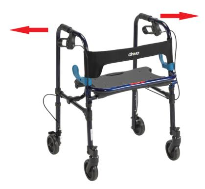
2. Each leg has to be adjusted to the desired height. Push in the locking pin on the leg and twist the leg slightly. Slide the leg to the desired height and twist the leg back to engage the locking pin. Repeat this procedure for the remaining three legs. The walker is now ready to use.
