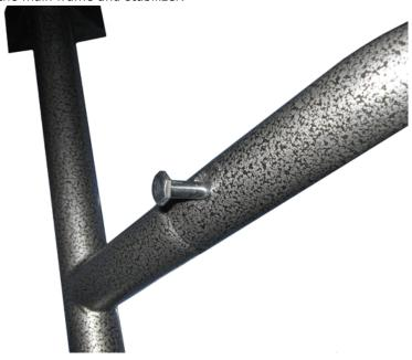
4. Make sure the bolt is pushed into the six sided cut out in the main frame.
