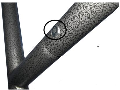
5. Install the one of the cove washers on the bolt with the concave side facing the main frame.
