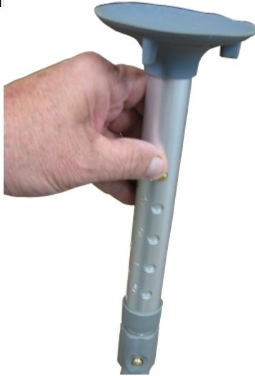
7. Adjust the leg by pushing in the locking button and turning the leg slightly. Slide the leg to the desired height and turn back until the locking button snaps into place. Repeat this process for the remaining legs.
