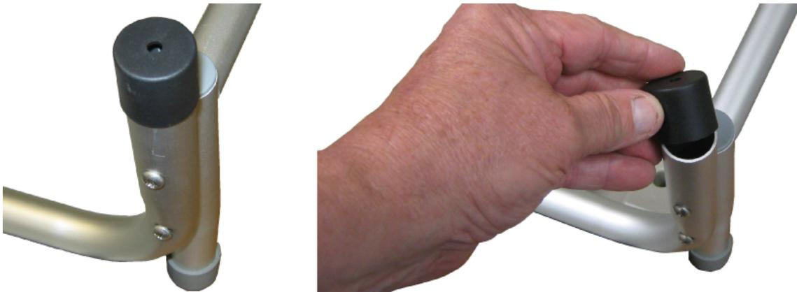
3. Install each leg into the receiver by depressing the locking pin and sliding the leg into the receiver. Make sure the locking pin engage into the receiver. Install the inner legs into leg receivers in the side of the base with two cushions on it. Install the outer legs into leg receivers in the side of the base with one cushion on it.
