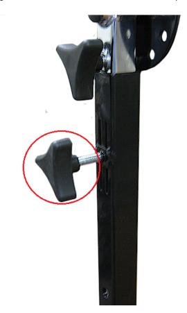
9. The lower mast can be set at either 45 or 90 degrees to the floor. To change the angle, loosen the lower base locking knob by turning it counterclockwise. Move the mast to the new position. Lock the lower mast in place by turning the knob clockwise.
