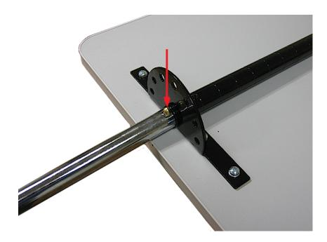
6. Make sure the lower mast is set at 90 degrees. If it is not, loosen the upper base locking knob by turning it counterclockwise. Set the upper mast at 90 degrees to the table top. Lock the lower mast in place by turning the knob clockwise.
