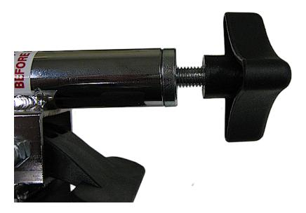
8. Align the locking wedge and mast tube with the end of the table mounting bracket side that is closest toe the table edge.
