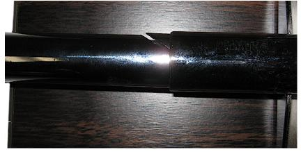
9. Side the mast all the way into the mounting bracket.
