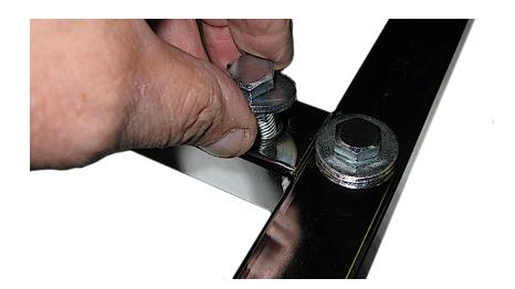
13. Align the holes in the base with the bolts.
