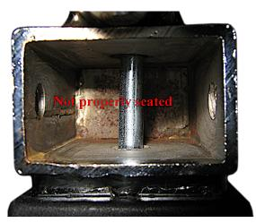
3. Insert the trip lever with the curve part facing up..
