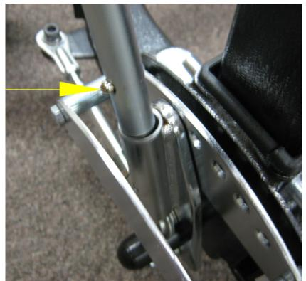
8. Make sure the nuts are backed off from end of the handles and then screw both push handles into the mast. When the push handle are screwed in as far as they will go tighten the nuts to lock the push handle on the mast.
