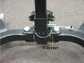
6. Install the two sets of bolts and washers that were previously removed through the base into the mast. Tighten both with the wrench provided.
