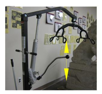
15. To lower the boom, turn the release lever slowly counter clockwise until the boom starts to go down.
