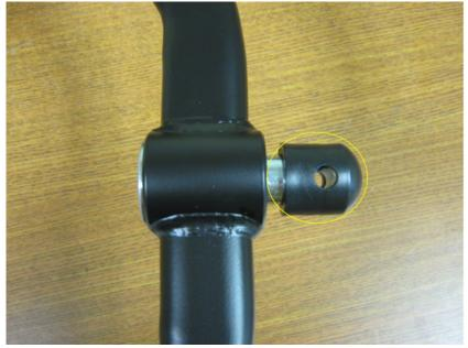
11. Align the holes in the "U" bracket on the boom and with the holes in the pivot bolt with cap. Insert the bolt from the cradle hardware through the "U" bracket and pivot bolt with cap.
