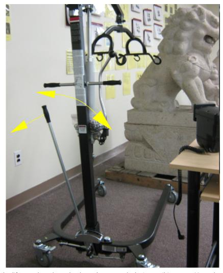
14. To raise the boom of the lift turn the release knob on the pump clockwise until it stops. Move the handle on the pump up and down until the desired height is reached.
