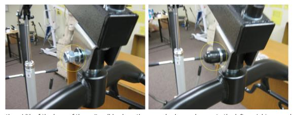
13. To change the width of the base of the unit pull back on the spreader bar and move to the left or right as needed.
