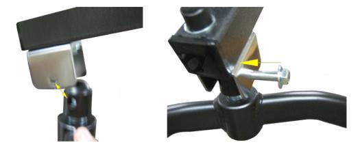
12. Install the second washer and nut onto the bolt. Install the nut cap unto the nut. The unit is nowready to use.
