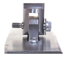
3. Slide another 10mm washer over the bolt and thread on and tighten a 5/16" locknut.
