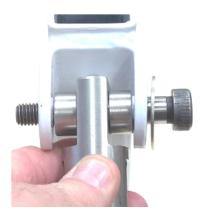
7. Add a 10mm flat washer, and then thread on and tighten a 12mm locknut.
