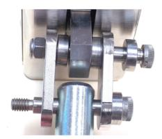
11. Slide a  $\frac{1}{4}$ " spacer over the protruding bolt, and install and tighten a  $\frac{5}{16}$ " locknut.
