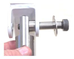
5. Next, slide another 12mm spacer onto the bolt.
