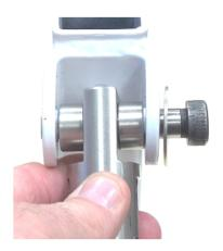
6. Now, push the bolt through the second hole in the lift arm.
