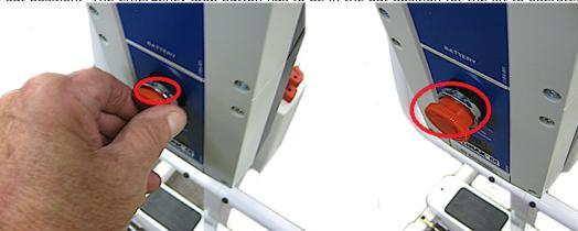
15. Insert the spreader bar into the receiver plate and depress the locking button. Continue to insert the spreader into the receiver plate until it locks into place
