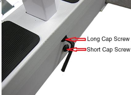
6. Remove the Allen cap screw from the upper and lower push handle posts with the Allen wrench provided.
