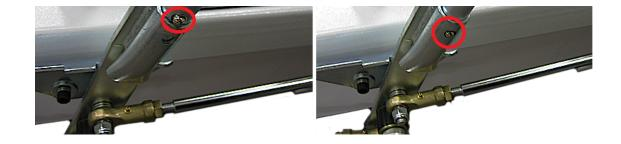
16. Insert the cradle swivel pin and nylon washer into the cradle.
