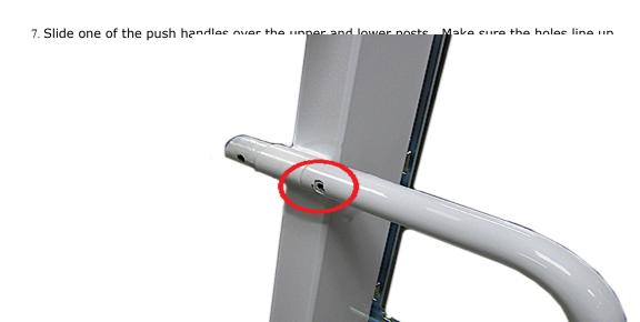
8. Install and tighten one of the Allen caps screw that were remove in the upper and lower push handle post. Repeat steps 7 and 8 for the other side.
