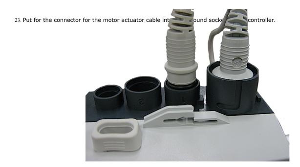
24. The plug must be pushed in flu amount of petroleum jelly on the
