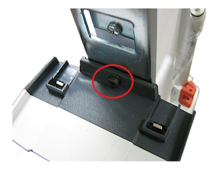
11. Line up the battery pack with the control box.
