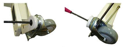
3. Turn the wrench counterclockwise to remove the nut and the wheel will come off. Reverse this procedure to install the replacement wheel.
