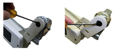
2. Use a 6mm Allen wrench on the head off the bolt and a 17mm socket or wrench on the nut.
