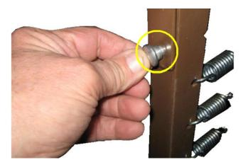
4. Install the nut and tighten.
