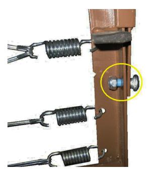
5. Install the lower frame extension on the head end of the bed frame..
