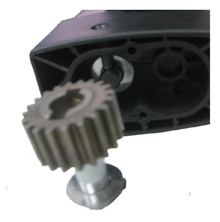
9. Slide a flat washer, a wafer bearing and then a flat washer over the shaft of the thin gear.
