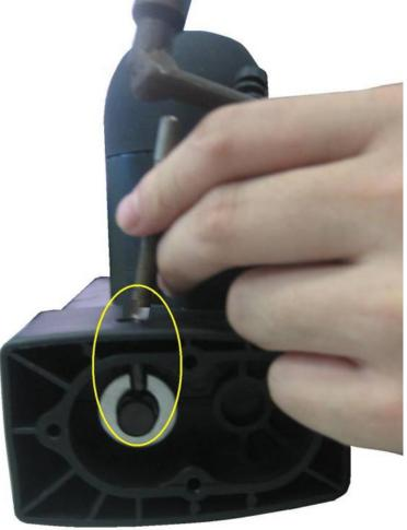
8. Install the thick gear over the short shaft of the motor. Verify that the thick gear seats completely flush with the flat washer. If it does not reposition the roll pin to accomplish this.
