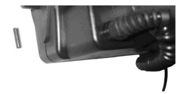
4. Slide the motor adapter over the short motor shaft.
