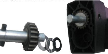
10. Install the thin gear with washers and wafer bearing into the motor adapter. Find a position so that the roll pins of both gears are as close to parallel as possible.
