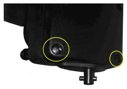
3. Remove the roll pin from the short shaft of the motor.
