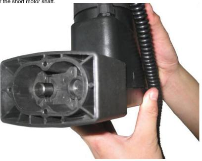
5. Install the two long screws through the motor adapter and tighten to secure the motor adapter to the motor.
