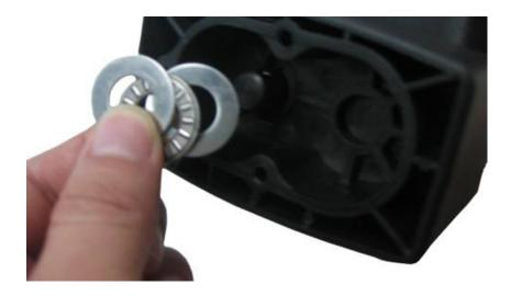
7. Install the roll pin back into the short motor shaft. Make sure the roll pin is in front of the washers and wafer bearing that was installed
