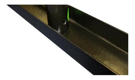
14. Align the hole in the pole assembly with the hole in the H bracket and install a locking pin.
