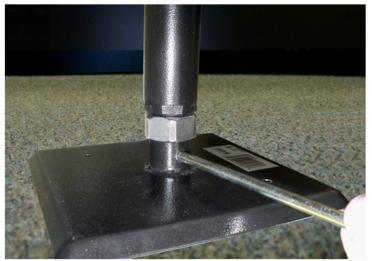
19. Turn the rod, driving the adjustment screw until the pole is slightly wedged between the floor and ceiling. Re-check for plumb of the pole and alignment of the holes on the H ceiling bracket and then turn the rod additional turns to tightly wedge the pole between the floor and the ceiling.
