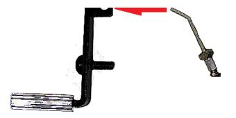
4. Install the cable fastener and test the brake. If the brake is too tight, loosen the cable fastener, apply the brakes slightly and tighten the cable fastener. If the brakes are not holding, loosen the cable fastener and pull more of the cable through the fastener and tighten the cable fastener. Final adjustments are made with the cable adjuster.
