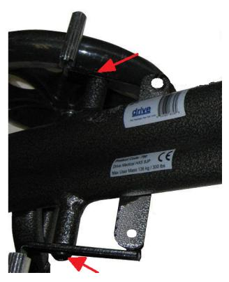
2. Remove the cable fastener from the brake cable.
