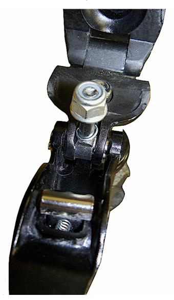
6. To remove the spring, loosen the column locking Allen head screw.
