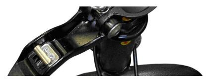
7. Remove the tiller from the steering fork.
