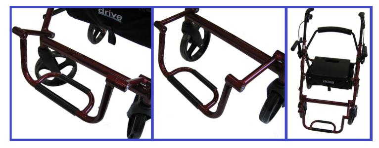
9. To adjust the length of the foot rest push in the locking pins and slide the down tubes of the footrest up or down to the desired length. Be sure the locking pins engage at the new length. To fold the foot rest back in to the Duet frame, the foot rest must be in the highest position.
