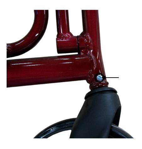
2. Tighten the bolt slightly. Try the rollator, if the flutter still exists, tighten slightly again.
