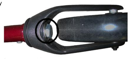
3. When the flutter is gone tighten the Allen screw.
