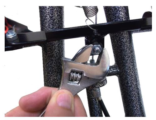
3. Pull the cable through the lock nut.
