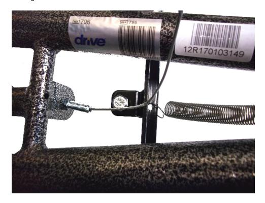
4. Disconnect the cable from the lever by pulling the sleeve out and guiding the cable through the slot in the lever.
