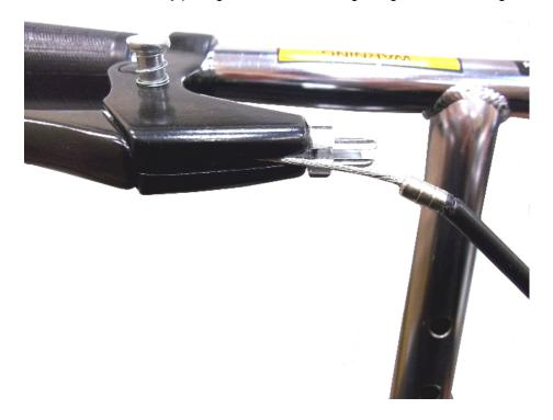
5. Pull the lever and expose the cable end, and slide the ferrule out of the retainer
