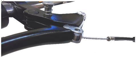
4. Thread the cable through the slot in the lever, making sure the sleeve remains in the adjuster seat.
