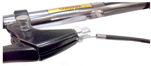
5. Now go back to the cable end at the brake, and, using pliers, pull the cable tight, and, while holding tension, tighten the retaining nut.
