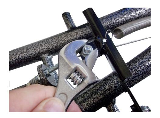
6. If necessary, the brake can be adjusted at the bottom threaded adjuster,
