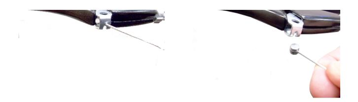
6. Pull the cable sleeve out of the guides (3).
