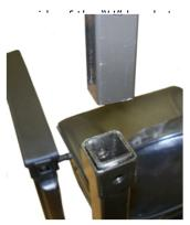
15. Align the hole in the "L" support bracket with the hole in the "U" bracket and install a nut and bolt. Tighten the nut
