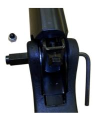
11. Slide the "U" bracket until the hole in the armost bracket aligns with the threaded hole in the extended nut.
