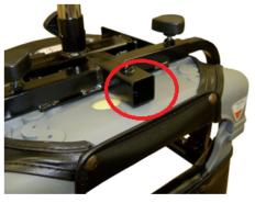
4. Slide the SF8050 mounting bar into the accessory mounting bar and screw in the locking knob. Do not tighten the knob. The SF8050 mounting bar should be able to slide back and forth.
