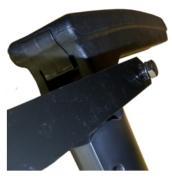
13. Repeat steps 9 through 12 for the other side. Tighten all the bolts and nuts and knobs. Install the seat on to the scooter.
