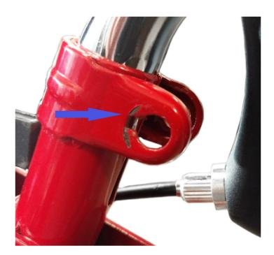
3. Insert bolt into clamp from the seat side of the frame.
