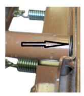
6. Remove the actuator bar from the frame.
