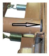
8. Place the separator between the actuator bar and the frame tilt bar. Replace the screw and nut. Tighten the screw and the nut and then back off a quarter of a turn. Repeat for the other actuator bar. Assemble the bed and verify there is no binding on the bars, loosen as needed.
