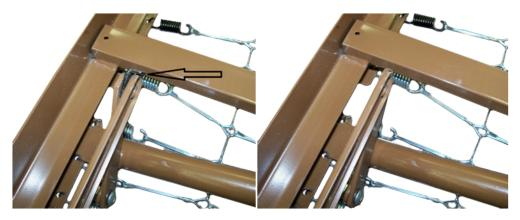
4. Using the 6mm Allen wrench remove the cap screw holding the actuator bar to the side frame of the bed.
