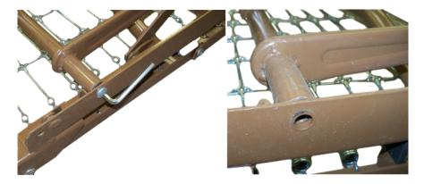
5. Remove the nylon washer from between the actuator bar and the side frame. Repeat steps 4 and 5 for the other side.
