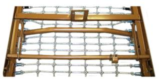
2. Using a 6mm Allen wrench and a 17mm wrench remove the nut and cap screw from the actuator bar and frame tilt bar.
