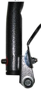
2. Lightly grip the pin end of the locking pin with a pair of pliers. Place a wrench on the nut side of the locking pin.
