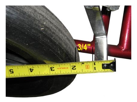
4. The wheel should not turn when set correctly. If it still turns adjust the brake closer to the tires. If the brake it is extremely difficult to engage the brake, move the brake further from the tire. WHEN THE BRAKE IS PROPERLY ENGAGE THE TIRE CAN STILL SLIDE ON THE FLOOR.
