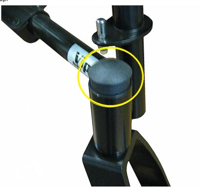
2. Flip the chair on its back. Remove the fork stem nut and remove the fork.
