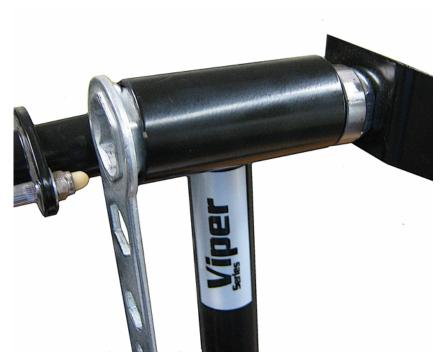
3. Install the new fork through the caster housing. Install the fork stem nut and tighten. Do not over tighten the fork
