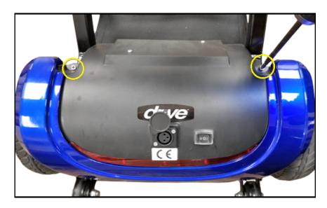
2. Turn scooter on side and locate two screws on the underside of the rear shroud and remove (or loosen enough to gain access to the back up alarm)
