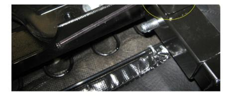
10 Slide the ELR bracket into the mounting bracket. The mounting pins on the ELR bracket have to be on the out side of the seat and '
