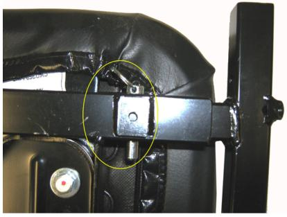
8. Insert one of the Allen-boad set scrows into the adapter bracket
