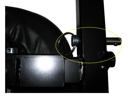
12. Install one of the locking knobs into the nut welded on the mounting bracket. Tighten the knob until the ELR bracket is locked in
