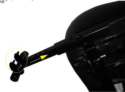
11. Align the hole in the mounting bracket with one of the holes in the ELR bracket. Insert one of the grenade
