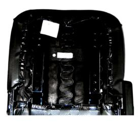
3. Place the seat plate on top of the adapter bracket. Align the holes in the seat bracket, the adapter bracket and the seat. Install the four bolts that were removed in step 1 using a 13mm wrench or socket.
