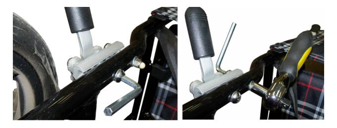
2. Slide the brake down a small amount. Tighten the mounting bolts and test.
