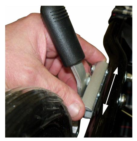
If the is to tight repeat step 1 and move the brake up. If the brake still does not engage repeat steps 1 and 2. If after the brake is moved as far down as possible and still does not engage, it is time to replace the rear wheel.
