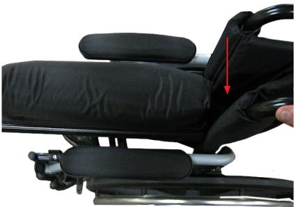
2. Push down on the rear section of the cross brace that is nearest to you with the heel of your hand. Have you fingers facing toward the middle of the seat upholstery. Do not put your fingers under the cross braces.
