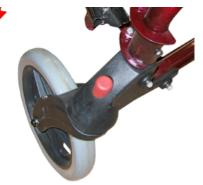
4. Continue to swing the footrest to the inside of the wheelchair until the release lever locks into place.
