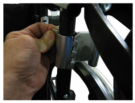
5. Insert one carriage bolt through the main body of the front anti tipper and then the hinge clamp bracket. Put the cap nut on and hand tighten. Repeat this procedure for the other carriage bolt and cap nut.
