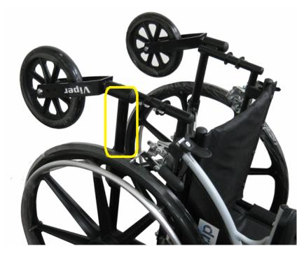
3. Each front anti tipper is mounted on the outside of the wheelchair. Position and hold the main body of the front anti tipper against lower frame of the wheelchair.
