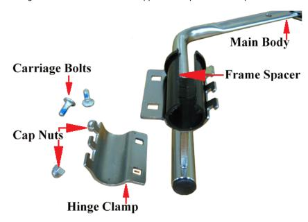
2. The front anti tippers are installed on the lower side frame just behind the casters. The frame spacer is used on narrow diameter frames. Turn the wheelchair on its back and install the frame spacer if needed.
