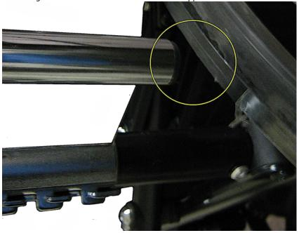
7. Inspect the hinged triangle has clearance of 1 inch off the floor. If there is not enough clearance move the hinged triangle to the second hole. When the correct position is set tight the cap screw that the Hinged triangle swivels
