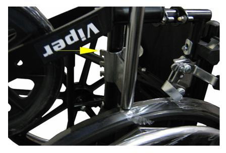
4. Install hinge clamp bracket onto the main body of the front anti tipper and hold in place.
