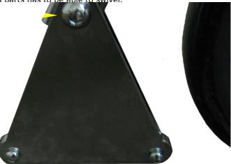
8. Verify that the front caster will not hit the front anti tipper when the fork is turning. If the caster does hit the front anti tipper then slide the front anti tipper back. When all clearances are verified, make sure that the front anti tipper is perpendicular with the ground and tighten both carriage bolts.
