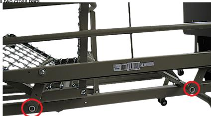
9. Install a washer and a nut on the end of both cross. Do not over tighten.
