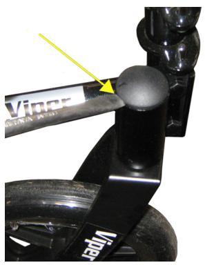
10. Remove one of the fork stam nuts and remove the fork and caster. Persont for the other fork and caster.
