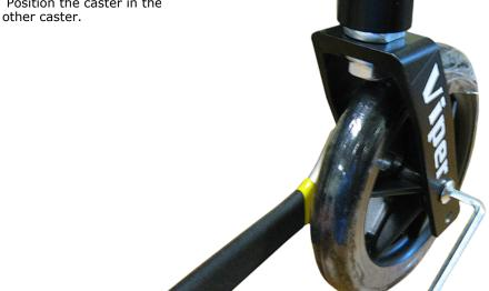
14. Slide the brake shoe extender over the brake shoe with the Allen screws facing down and tighten with the Allen
