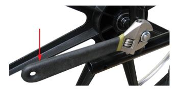
5. Turn the chair on its front side and remove one of the rear wheels by removing the rear axle.
