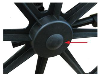
4. Remove the rear axle nuts from the rear wheels.
