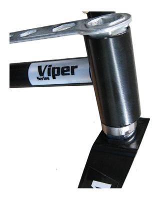
11. Install one of the new 6" casters and forks through the caster housing. Install the fork stem nut and tighten. Repeat for the other 6" caster and fork. Do not over tighten the fork stem nut. The caster and fork should swing freely, but not be k
