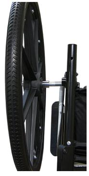
7. Install an axle nut on the new axle and tighten. The axle has to be held in place while tightening the axle nut to prevent the axle from backing out. Repeat steps 5, 6 and 7. Replace the two hub caps.
