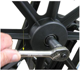
6. Install one of the new axles into one of the new 20" rear wheels and through one of the axle spacers. Install in
