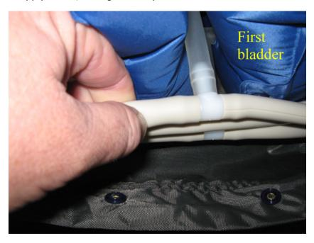
6. If there is no change in the firmness of the bladder, or they begin to deflate the leak can be found in either the bladder or the supply tube going to it.
