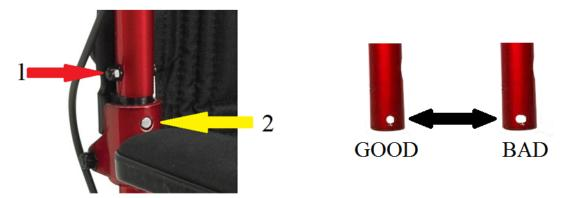
2. Verify that the locking pin extends all the way through the receiver. If it does not it can be adjusted by gripping the pin and turning the nut counterclockwise.
