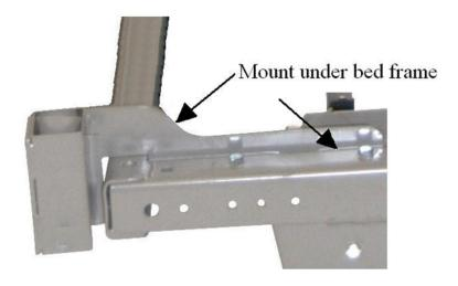
4. Install the lower bracket from the 15624 trapeze adapter kit in the center of the lower main frame of the head section. Have the clamps facing up
