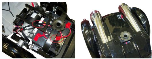
6. Screw the shroud back onto the frame. The small screws are used in the front of the shroud and the longer screws are used in the rear of the shroud.
