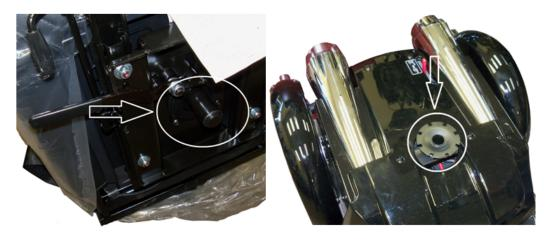
8. When the seat is seated on the frame pull the adjustment lever rearward and turn the seat back and forth to completely engage the seat on the frame. The seat should lock in place when the lever is released.
