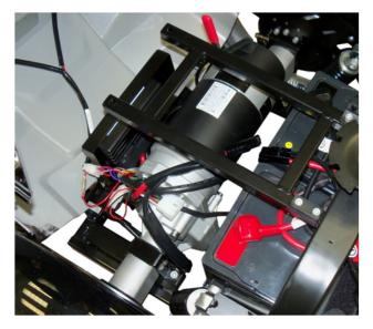
3. Locate the large red connector towards the front of the Maverick. It may or may not be connected. Connect by pushing both red connectors together.
