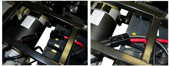
5. After both connections are connected place the rear shroud back on the rear frame.
