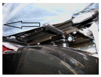
9. To install the headrest, align the two posts on the headrest with the mount on the back of the chair and insert into the mounts. Squeeze the adjustment lock and set the headrest to the desired height and release the button. Move the headrest up or down until the adjustment lock engages.
