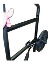
6. This will cause the inner sleeve to slide out of the frame and the cross brace can be removed. If the inner rail has rust on it spray WD-40 into the frame and let it seep down the frame and repeat step 5. Install the new cross brace in reverse.
