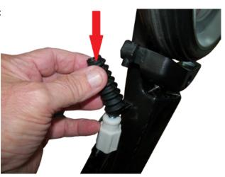
4. Pull cable through cable adjuster.
