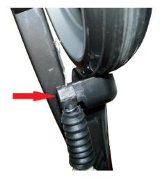
3. Remove spring and spring boot from cable.
