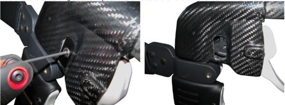
5. Pull the handle about 2 to 3 inches away from the handle. Remove the 2 silver bushings from either side of the brake handle.
