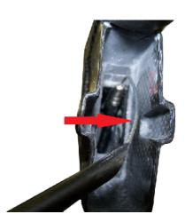
9. Push the end of the cable through the upper cable guide and remove the cable from the upper cable guide.
