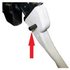
7. Pull the brake handle away from the housing being careful not to lose the small plastic cable pulley.
