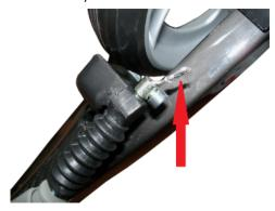
2. Loosen up the cable fastener with a 4mm Allen wrench and remove cable fastener from cable.
