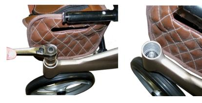
3. The screw that holds the hub cap on to the fork axle is either an Allen or a Torx head. Verify that the correct tool and size is being used as not to round out the head of the screw.
