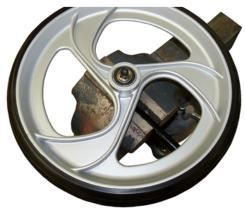
7. Gently tap down on the head of the screw until the "Tinnerman" nut is off the fork axle.
