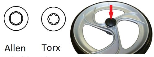
4. Remove the hub cap from the front wheel.
