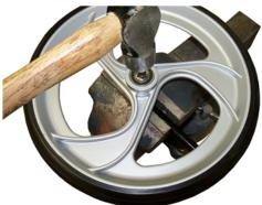
8. Remove the hub cap screw and the "Tinnerman" nut.
