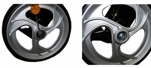
3. Using a 13mm socket remove the locknut from the axle.
