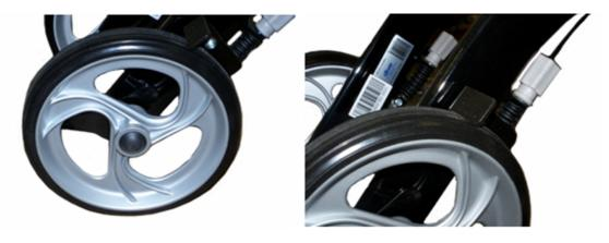
2. Using a small flat end screw driver pry off the hub cab.
