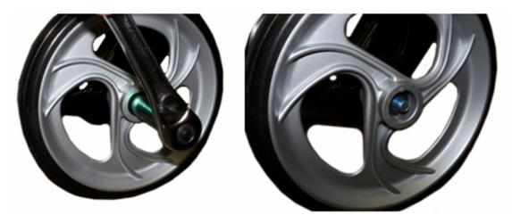
4. Release the loop brake and slide off the wheel. Install the new wheel following the  $\,$  steps 1 to 4 in reverse.
