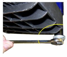
3. Grasp the footplate, turn the footplate loosen the down tube.
