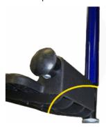
2. Loosen the bolt one or two complete turns.
