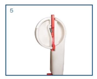
step 5 Remove spring and remove defective trigger.
