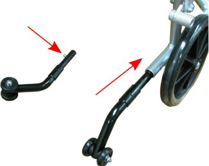
12. To disengage the anti-tippers, pull the anti-tipper rearward and swing 180 degrees until it locks in the upward position. Repeat for the other anti-tipper.
