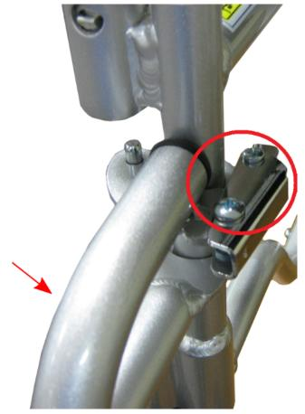
7. To remove the footrest, push the footrest release lever in and swing out the footrest.
