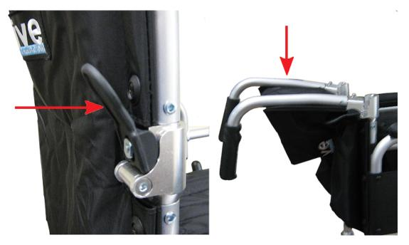
3. To unfold the chair grasp one of the handles and tilt the chair slightly. Push down on the top of the cross brace on the side of the handle you are holding.
