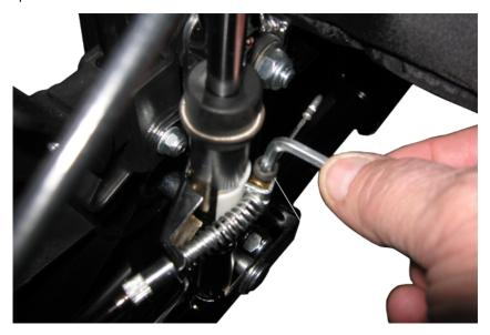
2. Pull and hold the cable tight. Make sure the cable stop is against the piston release bracket and tighten the cable stop.
