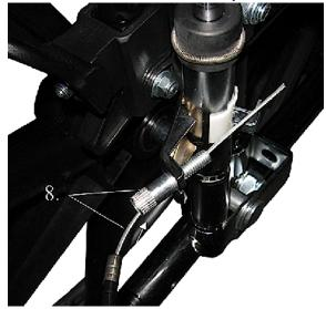
9. Install the spring that was removed in step 2 on the cable.
