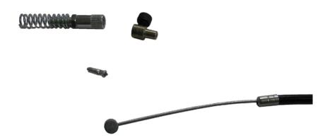
4. Thread the cable through the strain relief in the handle and then into the cable sleeve.
