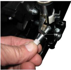
7. Mount the recliner release handle to the back can of the recliner.
