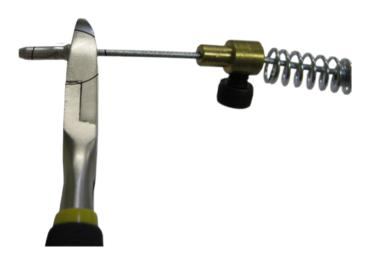
2. Remove the stop, spring and collar.
