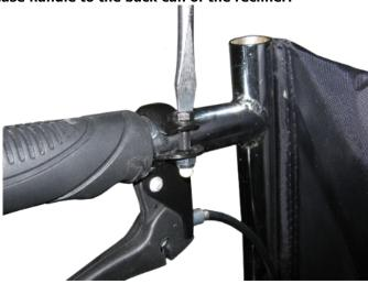
8. Insert the cable through the collar that was installed in step 6.
