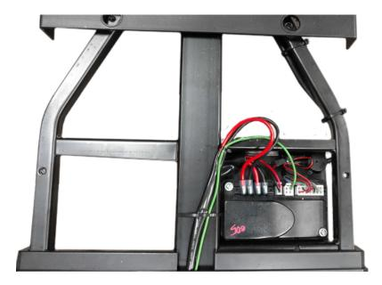
3. Unplug all connections, remove mounting screws (yellow arrow) using a #2 Phillips\* screw driver and remove controller.
