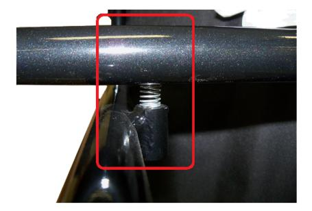
4. Remove the spring or spacer.
