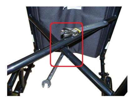
3. Check to see if there is a spring or spacer between the two sections of the cross brace.
