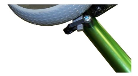
4. Place the rear bracket with the hole around the anti-reverse dowel nut.
