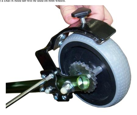
7. The knob on the top of the Dial-A-Speed Tab will adjust the resistance on the rear wheel or wheels.
