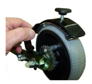
3. Lock the anti-reverse dowel in the disengaged position.
