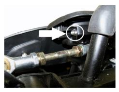
3. Using either a Phillips screw driver, a 5/16" ¼" drive socket with an extension or a 5/16" nut drive, remove the 2 screws holding the light to the light bracket. There is no need to use the new light bracket.
