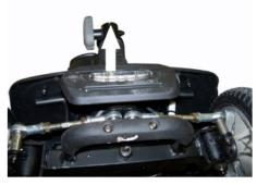
4. Remove the light through the front of the bumper shroud. Install in reverse with a new zip tie.
