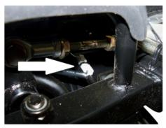
2. Cut the zip tie holding the light connector to the frame. Disconnect the light from the harness.
